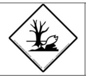
Packages and cargo transport units containing dangerous substances classified as "Marine pollutants" by the IMDG Code must bear the markings shown here and be durable. These should be placed close to the risk labels or risk placards of the goods. The dimensions of marine pollutant markings should be a minimum of 10 cm per side of packages and 25 cm per side of the pipeline and equipment used in that line.
